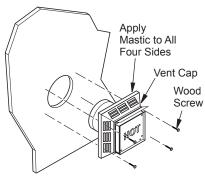
Figure 10 - Installing Horizontal Vent Cap (Noncombustible Exterior)
